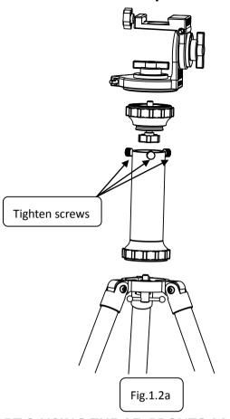
1.Loosen 3 screws on the side of the extension tube; take out the head piece of the extension tube; insert and screw it on tightly into the base of AZ PRONTO.
