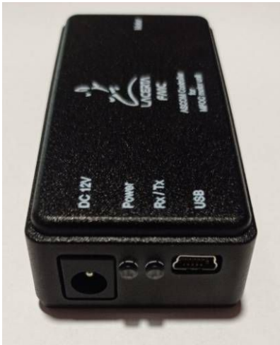
12V DC socket(5,5/2,1mm center positive) _ Power Led _ Serial Led _ USB-B mini and RJ45 to motor unit
