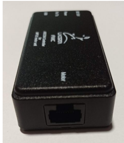
12V DC socket(5,5/2,1mm center positive) _ Power Led _ Serial Led _ USB-B mini and RJ45 to motor unit
