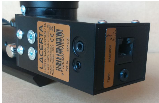
12V DC socket(5,5/2,1mm center positive) _ Power Led _ Serial Led _ USB-B mini and RJ45 to motor unit
